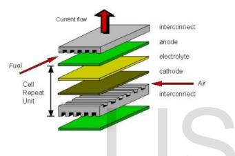
In the planar design, the components are assembled in flat stacks, with air and fuel flowing through channels built into the cathode and anode.
