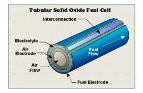
In the tubular design, components are assembled in the form of a hollow tube, with the cell constructed in layers around a tubular cathode; air flows through the inside of the tube and fuel flows around the exterior.
