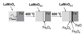
Figure 5. Scheme for the oxygen transfer from LaMnO<sub>3</sub> to Fe<sup>o</sup>, forming different iron oxide phases.
