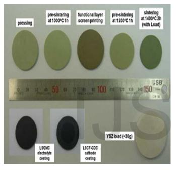
Fig: LSGMC electrolyte deposition at each preparation step.
