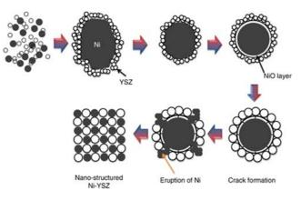
Fig: Formation of Nickel yttria-stabilized zirconia
