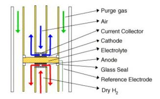
Fig: Components of Solid Oxide Fuel Cell
